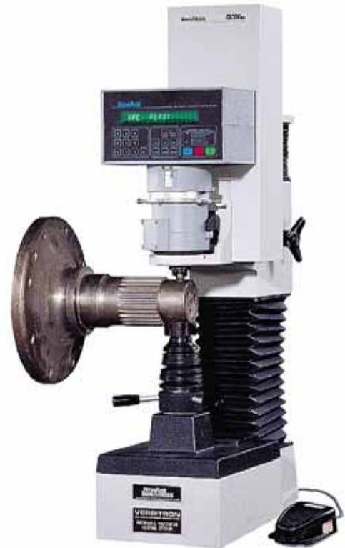
Heavy specimens exerting up to 240 foot pounds can be clamped in seconds. Above is an 80 pound spindle. Test results are unaffected since the stand, not the test head, bears the
